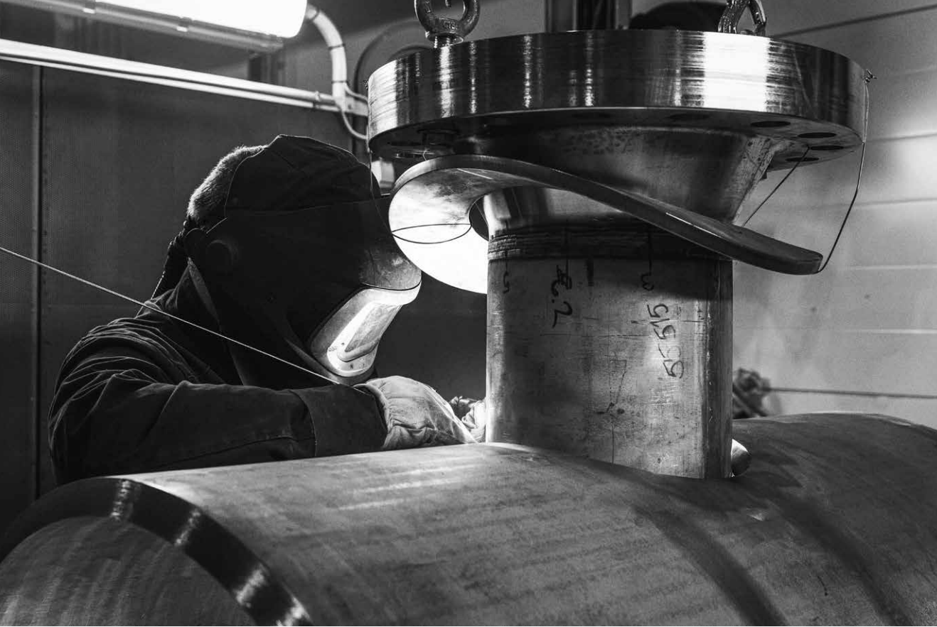
Saddle nozzle welding of pressure vessel, the shell specially made for each individual unit. Vahterus currently produces around 4,000 heat exchangers per year, which means an average of 90 units enclosed in their glossy white shells every week.
