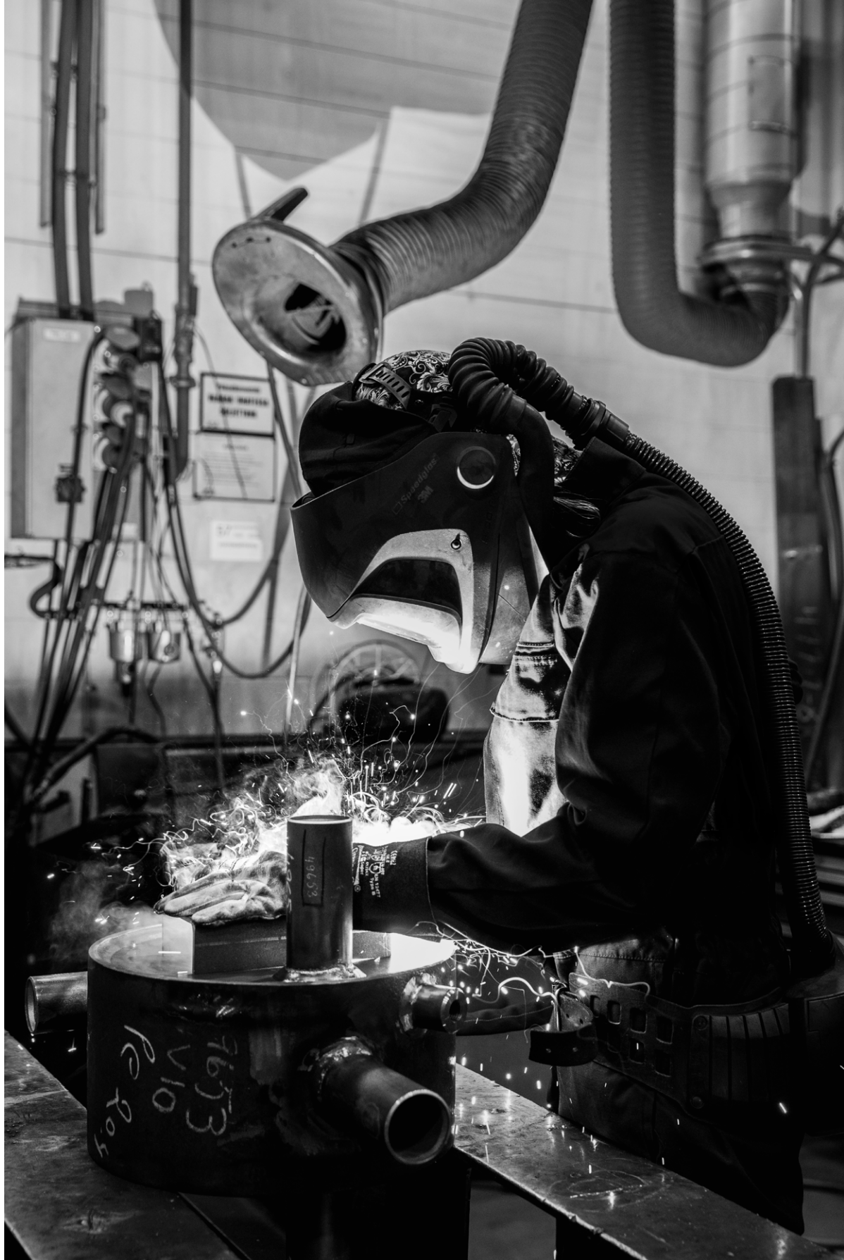
Welding of pressure vessel surrounding the plate pack.
