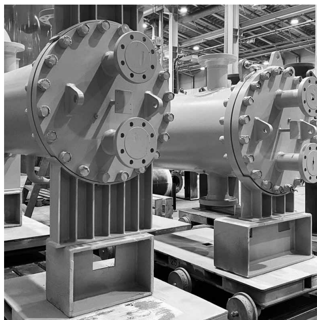
Vahterus heat-recovery units at a refinery whose waste-heat recovery system now heats around 150 industry buildings.
